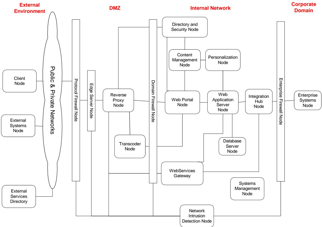
A detailed examination of each node in this diagram is outside the purpose of this document, but its inclusion here serves as a useful reminder of the many functions that must be considered when designing a modern IT infrastructure. Note, for example, the inclusion of three levels of firewalls as well as the “directory and security” and “network intrusion detection” nodes. The modern business climate demands a focus on security as indicated in this diagram.
