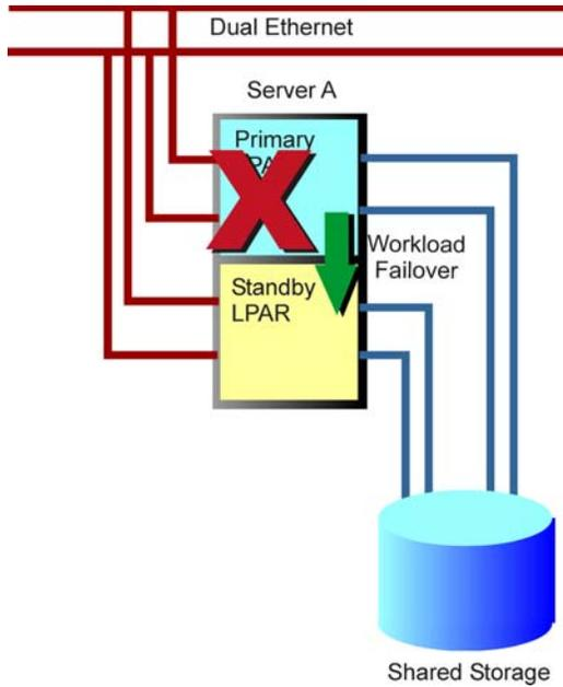
In the event of a failure in the primary LPAR, the workload will be failed over to the standby LPAR in the same manner that the workload failed over to the standby server in our classic 2-node cluster example.
