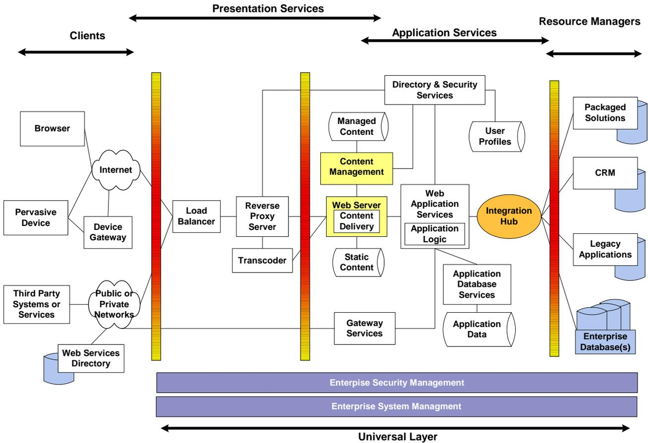
You can see how the “nodes” shown in the topology diagram are now replaced with indications of potential servers, workloads, and storage. The interconnections between the components suggest how the IP and storage networks might be designed.
