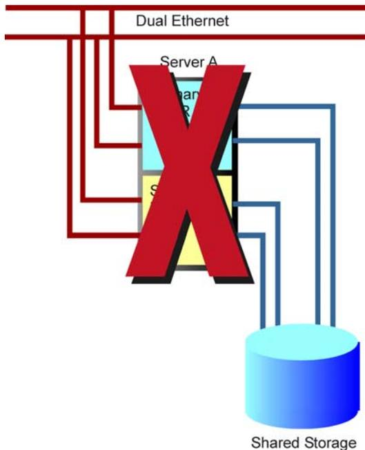
There is an issue with consolidating an HA cluster into LPARs on a single physical server. If the entire server fails or needs to be taken offline for a firmware upgrade, the HA cluster is unavailable until the server comes back up. This is a step backwards from the classic model with two physical servers.
