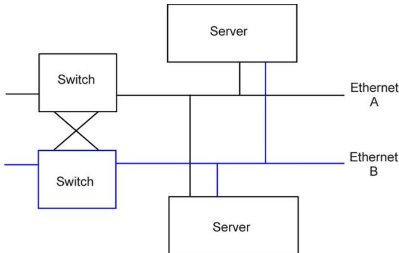
A further note about the server Ethernet connections: many Ethernet adapters now offer dual ports on a single adapter. Keeping the example diagram in mind, it is tempting to use one port on a single adapter for Ethernet A, while the second port is connected to Ethernet B. Be aware that this approach makes the
