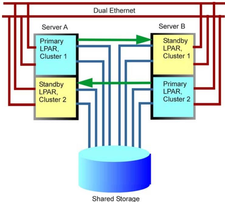
The resulting recommendation, then, is that you must plan for a minimum of two physical servers, even when using partitioned System p5 hardware. However, you can then define two or more 2-node clusters based on LPARs, with the primary and standby LPARs sited on different physical servers. Also, as shown at left, note how each physical server has one primary and one standby LPAR. This protects against the total loss of both primary and standby LPARs for a single cluster in the event of a
