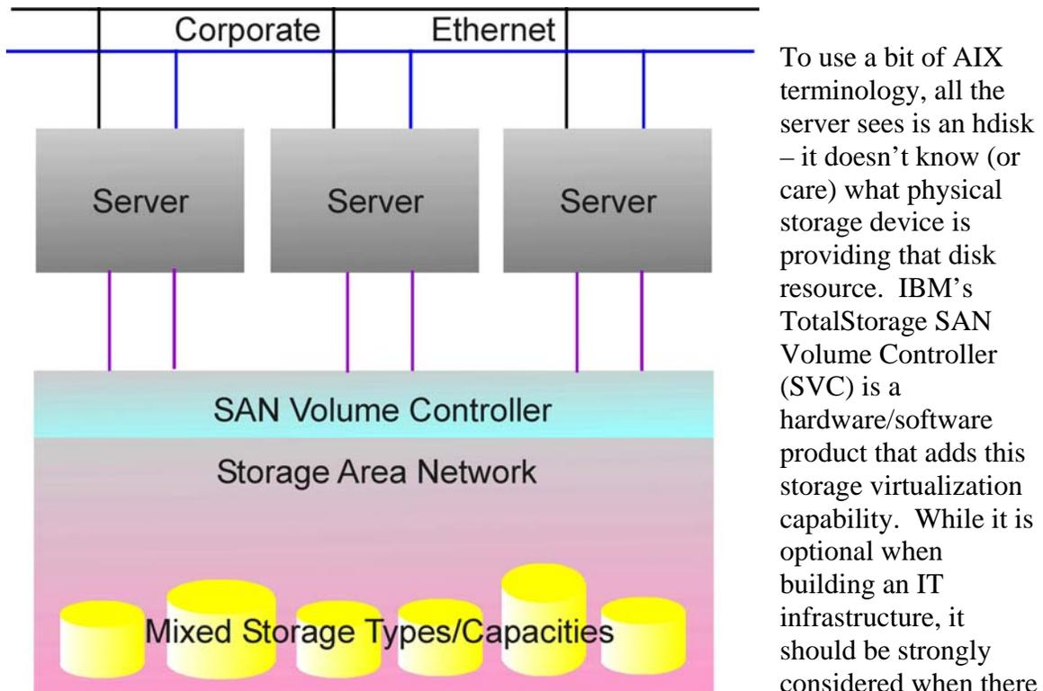
is a need for an adaptable, resilient storage infrastructure that can maximize the use of existing storage capacity across a mix of storage devices.
